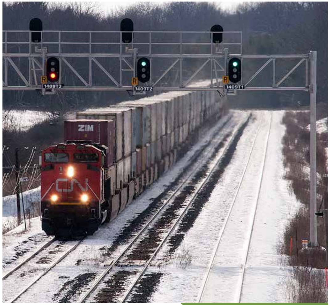
Intermodal freight trains provide a service that is faster than carload haulage through the substitution of truck pick-up and delivery for the equivalent rail processes required by traditional merchandise handling. Photo by Ray Farand
