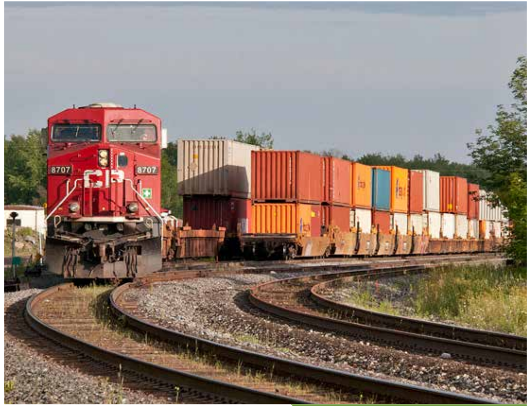
From trailers riding “piggyback” on flat cars in the early 1950s to today’s doublestacked containers moving in trains of 150 or more cars, intermodal has become one of the shining stars of Canadian railroading. Photos courtesy CP
