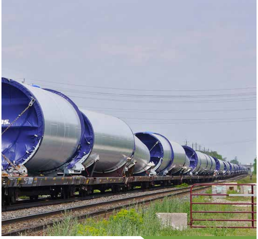
Oversized loads that can't be easily accommodated on the highways, such as wind turbine components (shown above), electrical transformers and industrial high-pressure vessels. Photo by Walter E. Pfefferle
