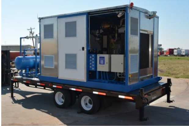
Figure 45 Mobile CNG Fueling Compressor Station
