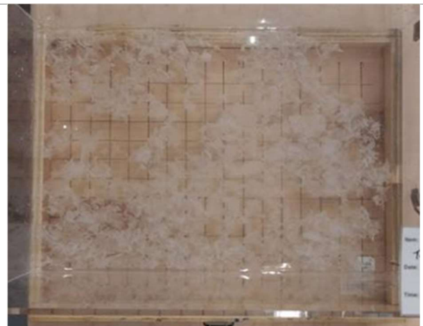
Figure 10- Example of Bathroom Tissue Disintegration After Testing
