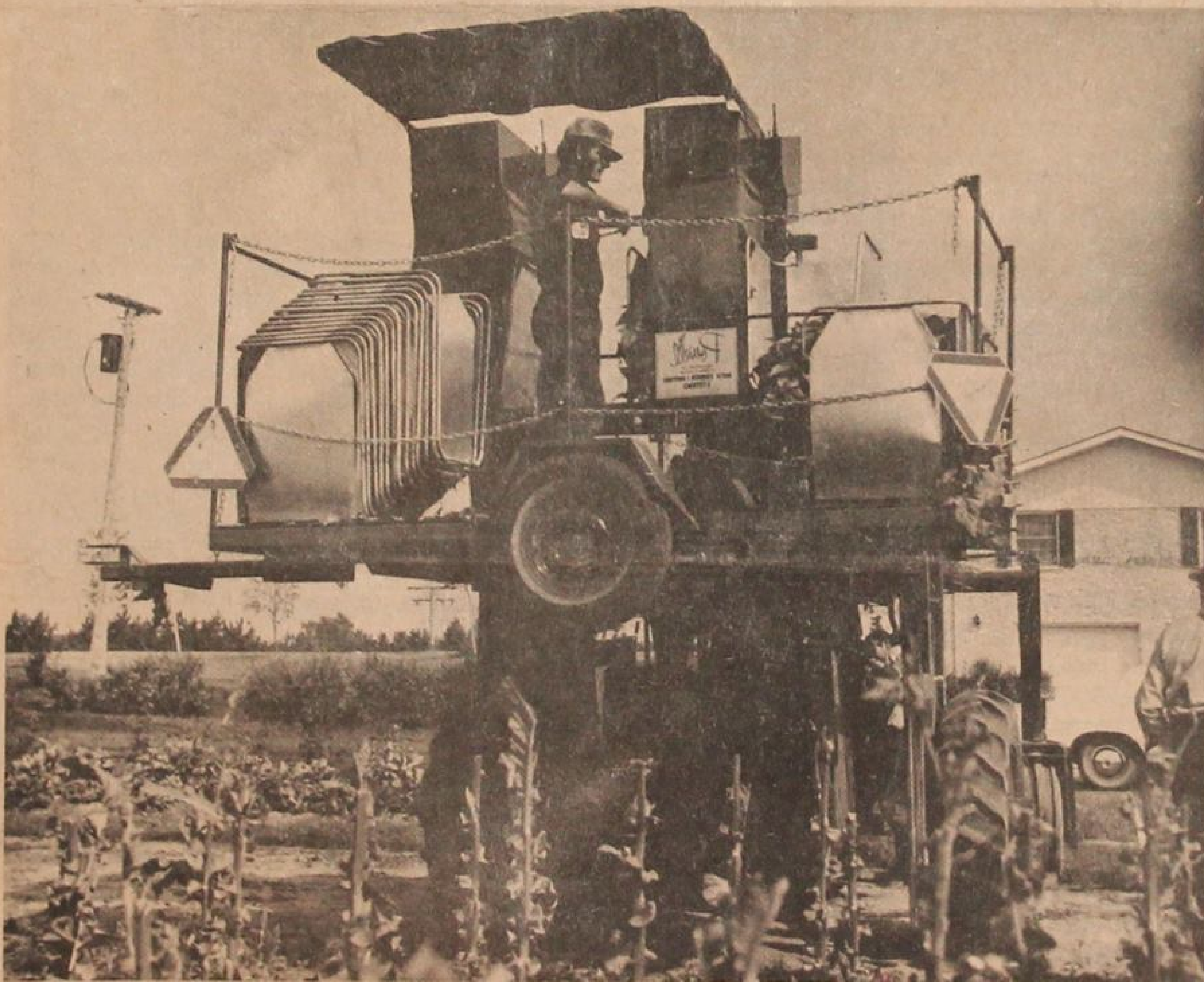
This newly developed harvester of the Powell Agri-Systems Ltd. of Otterville has an interesting feature. It carries along a trailer that is loaded with baskets of tobacco while the machine moves through the tobacco field. With hydraulic controls, the filled trailer is lowered to the ground and quickly replaced with another. (Art Goodwin)
