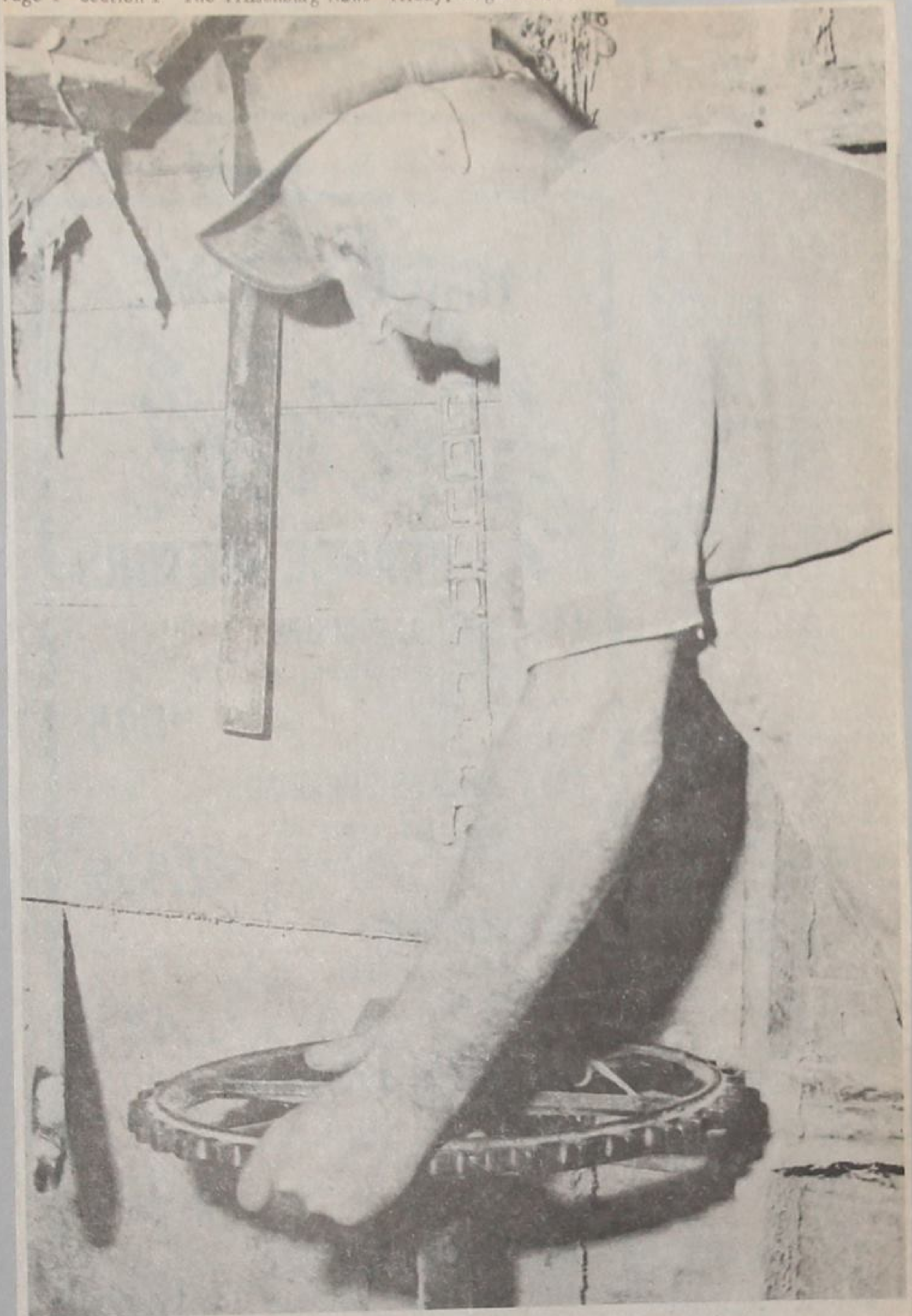
Mr. Treffry adjusts the flow of water which drives the mill's turbine.
