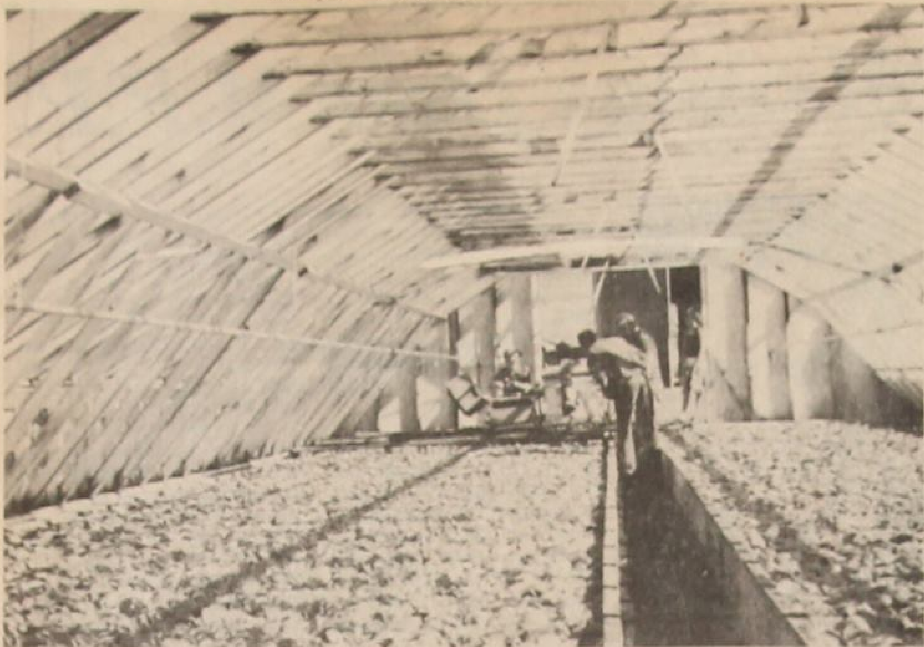
Set up on one side of the greenhouse, the plant puller moves along the side pulling only the plants big enough to be transplanted. A 100-foot greenhouse can be pulled in about three hours.
