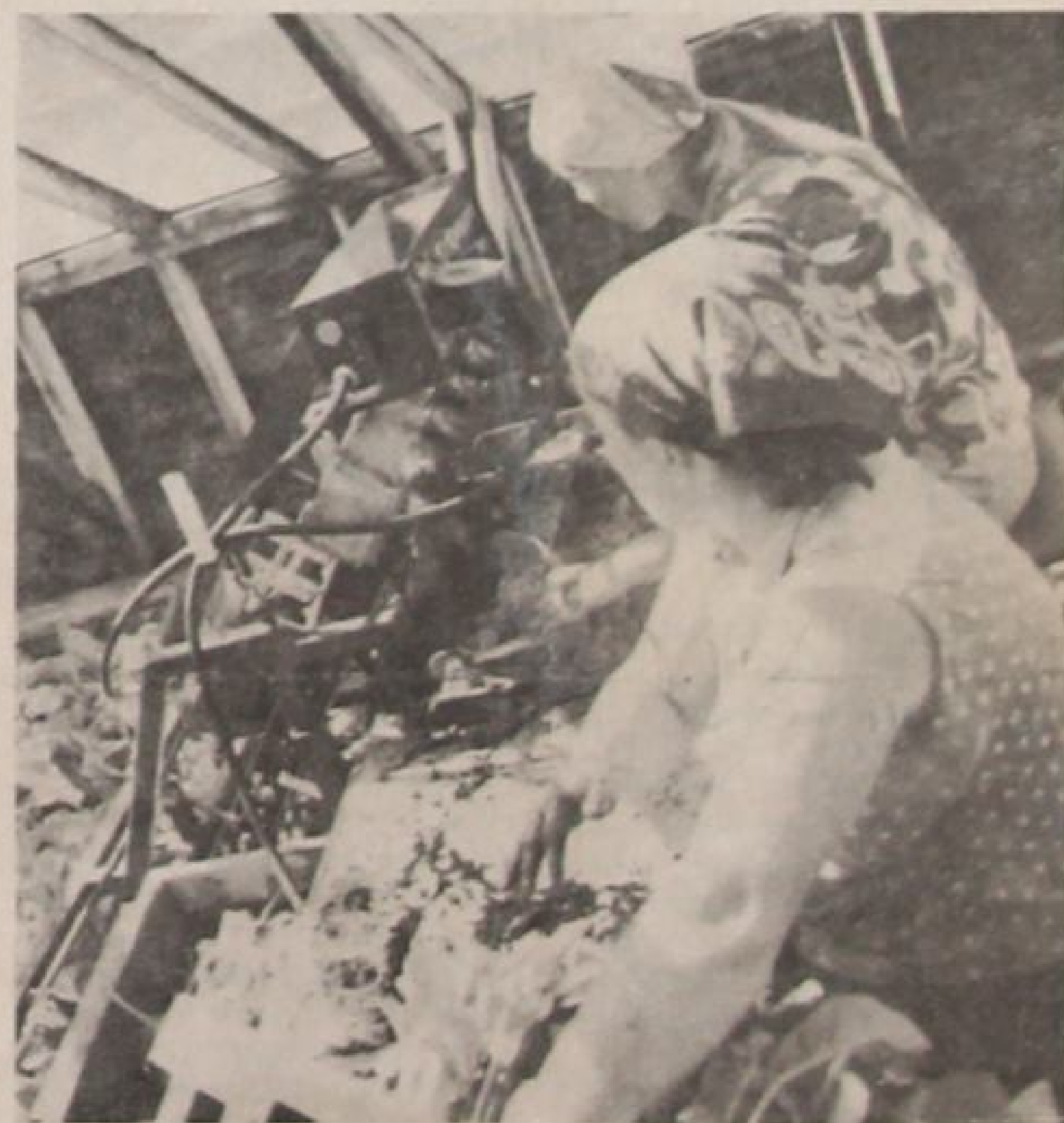
The controls of the plant puller regulate the speed with which it travels from one end of the greenhouse to the other, the speed with which the belts pull the plants and the minimum size of the plants to be pulled. The women operating it take the plants as they are dropped by the belts and place them in boxes to be transplanted.
