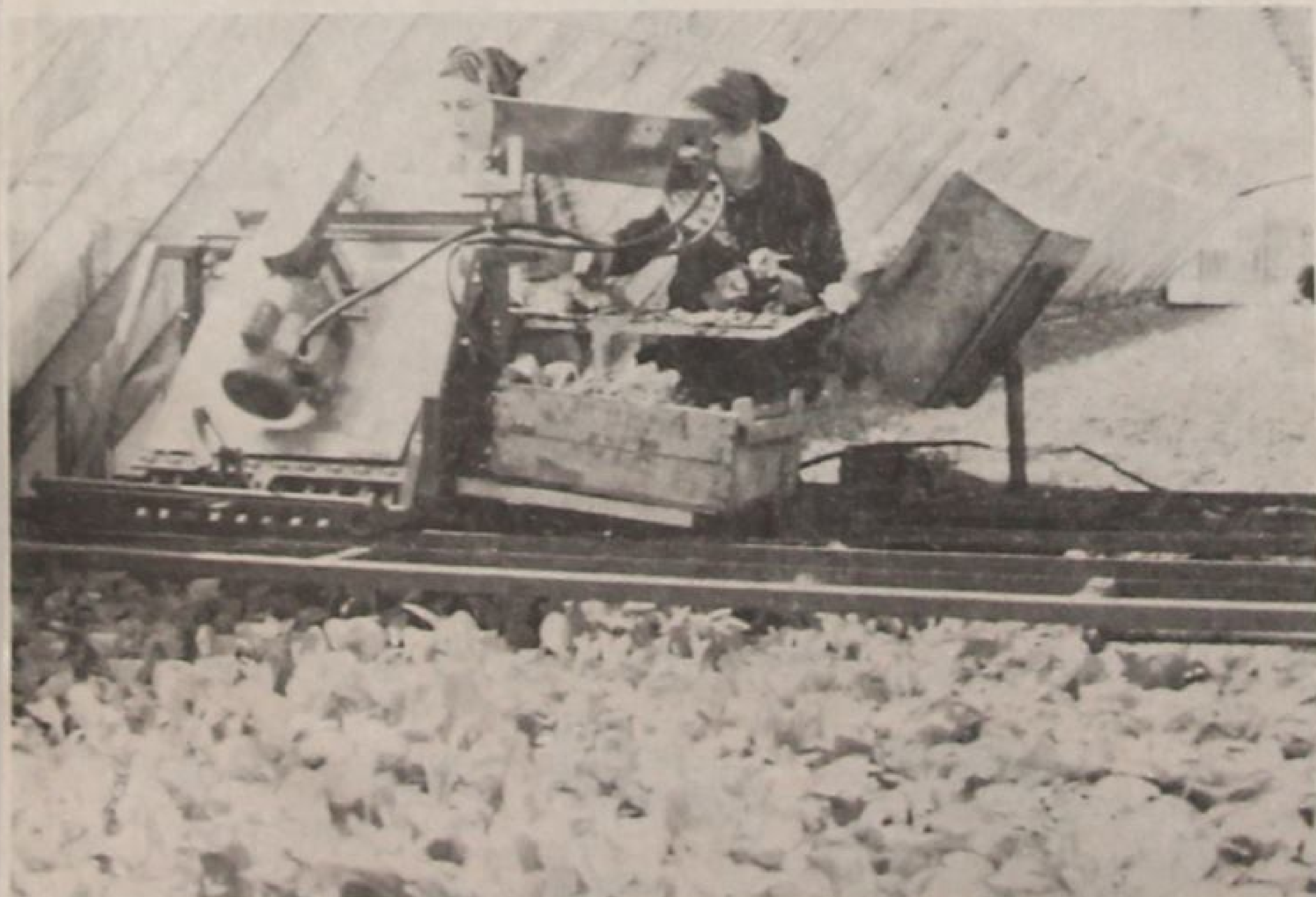
One or two people can operate the plant puller as it travels up and down the greenhouse.
