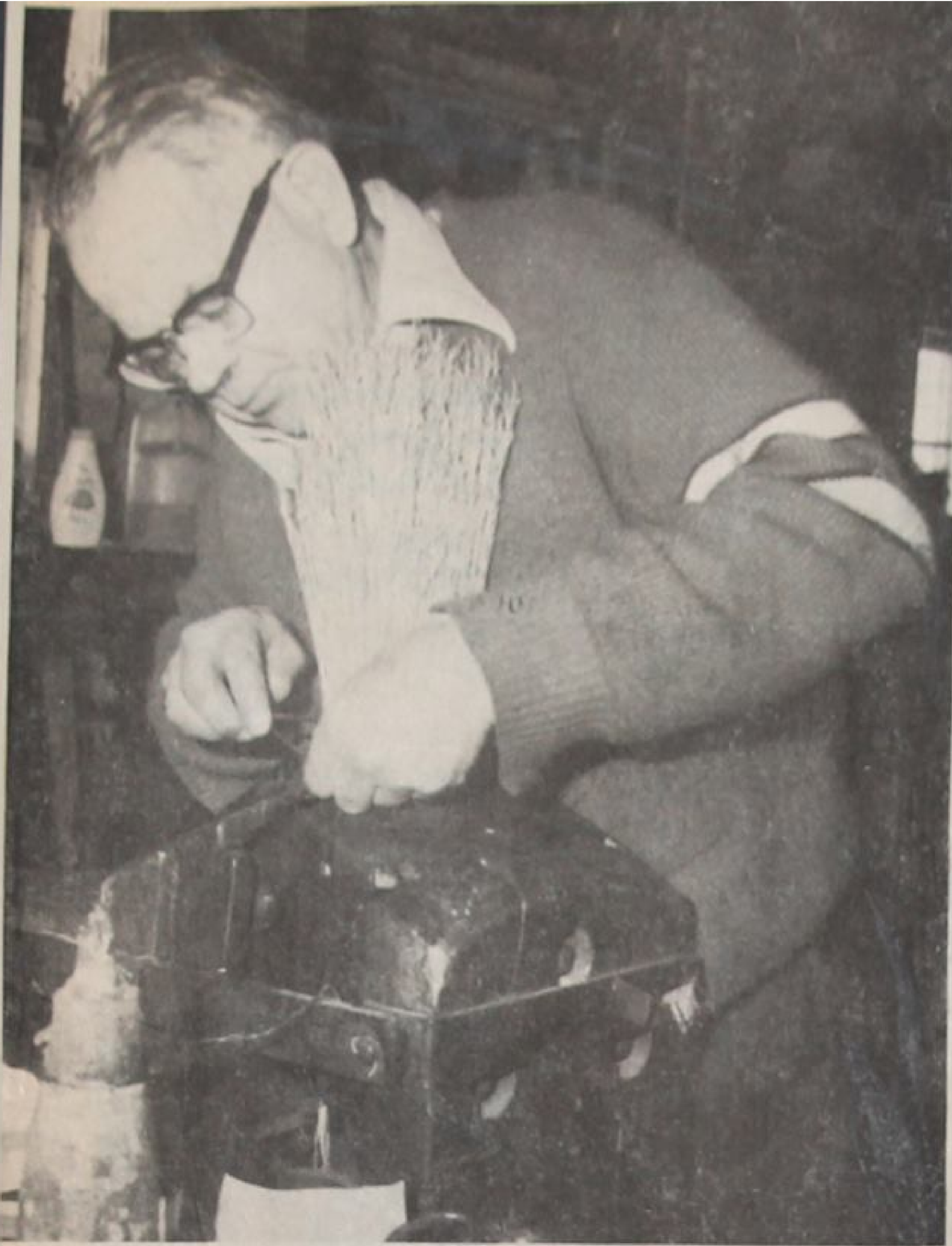
The second string is sewn onto the curling broom by hand, as Norm Lees of Norwich demonstrates. Mr. Lees started making house brooms in 1928 but now most of his business is devoted to curling brooms.
