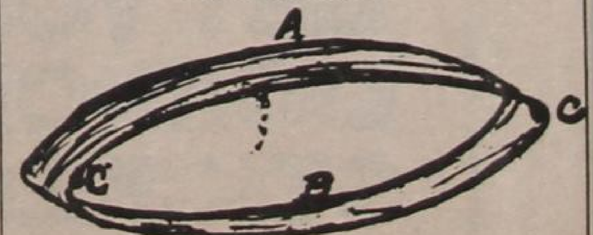
A THE UPPER LEAF B THE LOWER LEAF C BOLTS CONNECTING THE TWO LEAVES
